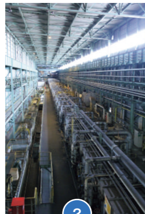
2 Annealing furnace (Horizontal radiant tube furnace)
