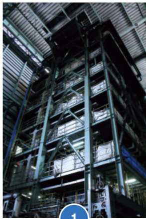
1 Annealing furnace (Vertical direct-fired reducing furnace)
